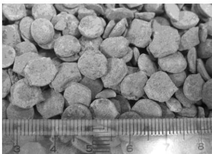
**Figure 4.** Product particles from wax-flake molding with a belt cooler (4020).
