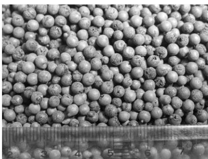
**Figure 3.** Spherical particles from new granulation process (4010NA).
